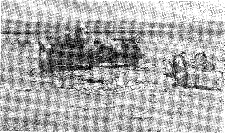
Figure 5.129a. Machine tools after a nuclear explosion (10 psi peak overpressure).
